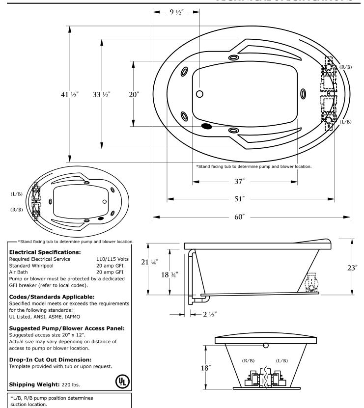
**Installation: Measure tub before building tub deck.** For best results, Jetta Corporation recommends 1''-3" of mortar bedding under the tub base for maximum support. Drawing shows manufacturer's standard pump location(s). Optional location(s) available at an additional cost depending on feasibility. Contact Jetta for details. Dimensional variance on drawings may be +/-1/2 inch and are subject to change without notice.
