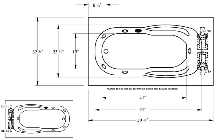
\*Stand facing tub to determine pump and blower location.
